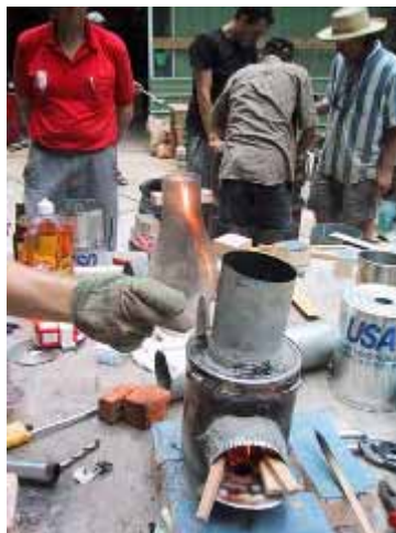
Dan trying to stabilize the burning pyrolyzed Gas in APROVECHO
